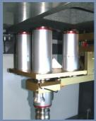
The machine is equipped with a motorized optical head which enables the laser spot size selection according to your chip dimensions.
