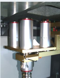
The machine is equipped with a motorized optical head which enables the laser spot size selection according to your chip dimensions. Moreover the advanced optical lenses ensure a homogeneous temperature on the all assembly area.
