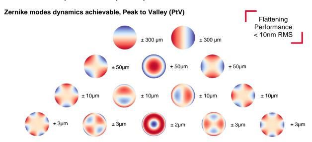
PtV dynamics are related to a diameter 80mm circular aperture with 35 actuators.
