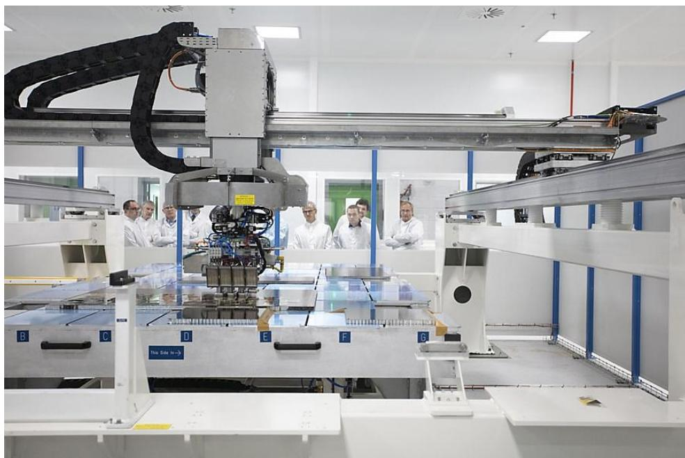
ISP System Cartesian robots are based on technologies developed since 1997 by our engineering departments. They fulfill high requirements in precision, rate and fiability expected by manufacturers.
