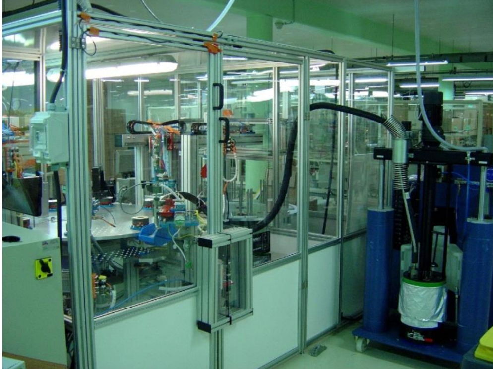
This machine assembles medical interfaces for ostomy pouch.
