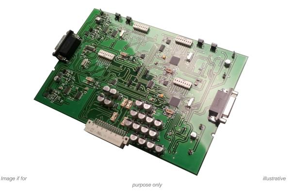
This board is a 4 axis motion controller for actuators using brush DC motor with optical encoder.
